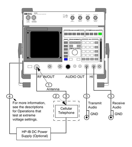
Figure 25 Equipment Connections
