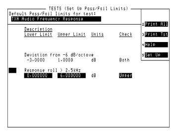
Figure 23 TESTS (Set Up Pass/Fail Limits) Screen
