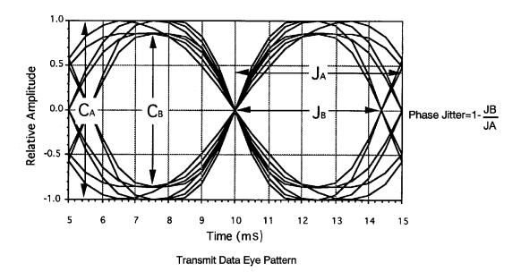
Figure 31 Transmit Data Eye Pattern, DSAT Phase Jitter
