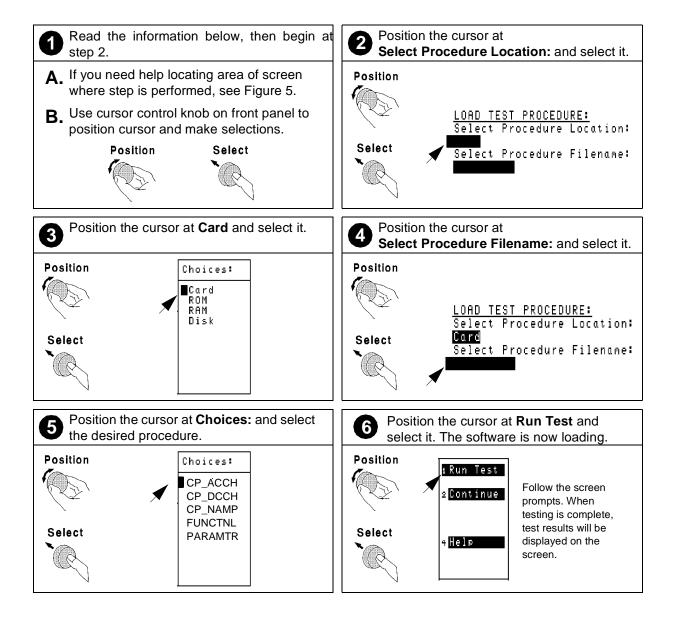
Figure 27 Selecting a Test Procedure
