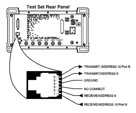
Figure 33 Serial Port Configuration
