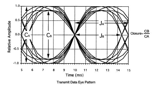
Figure 30 Transmit Data Eye Pattern, DSAT Closure
