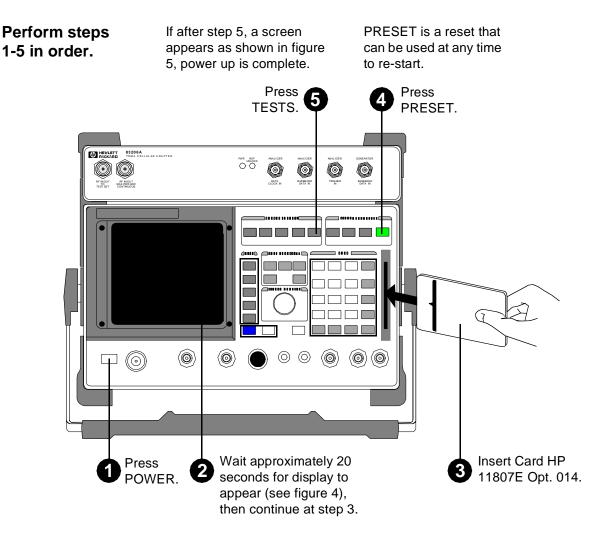
Figure 3 Setup and Software Loading Process
