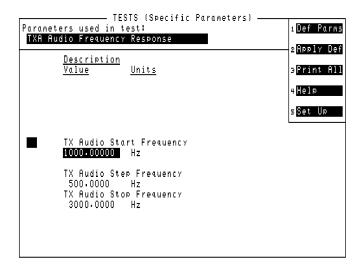
Figure 16 TESTS (Specific Parameters) Screen Showing Numerical Entry
