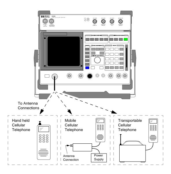
Figure 2 Equipment Connections
