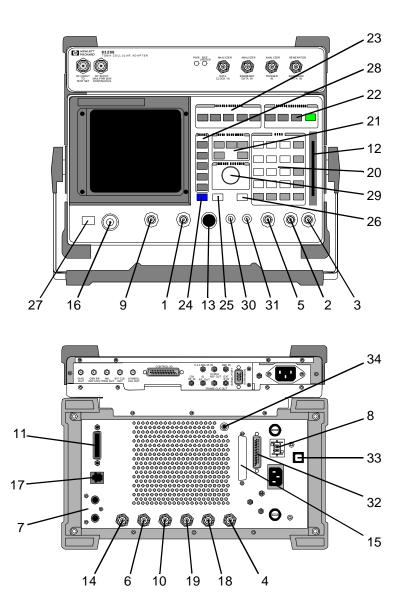
Figure 8 Test Set Connector, Keys, and Knobs
