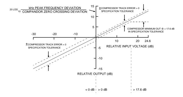
Figure 29 Compressor Curve
