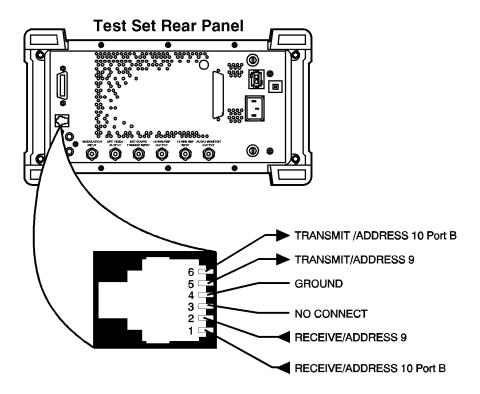
Figure 35 Serial Port Configuration
