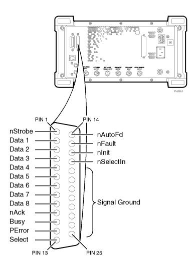
Figure 34 Parallel Printer Connections
